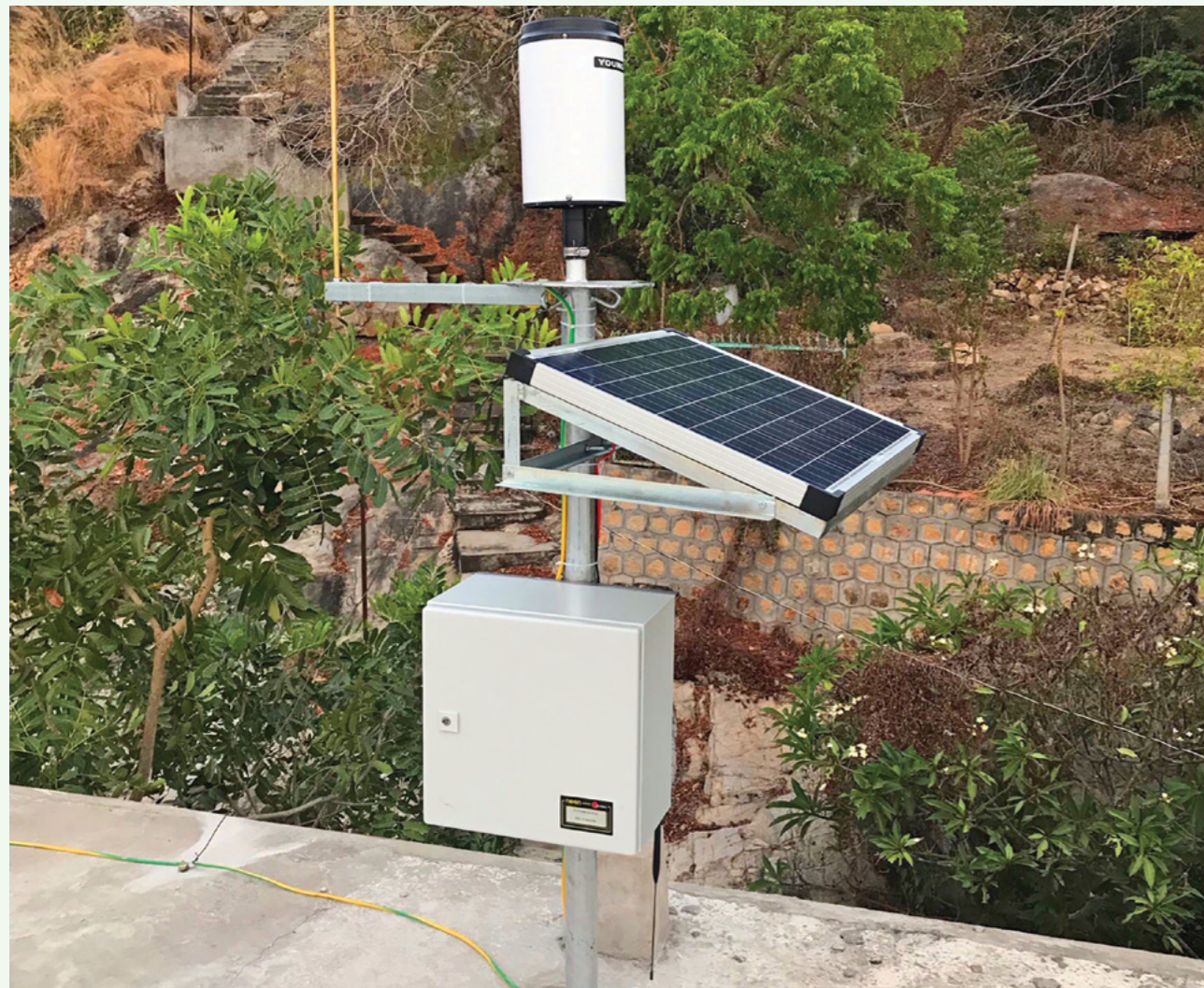
Automatic rain gauge at Hang Pagoda, Sam Mount, Chau Doc, An Giang Province, supported by GIZ Copyright © GIZ
