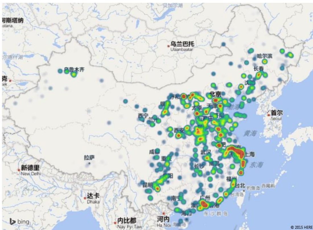
Figure 2-4 Distribution of power generation capacity of coal-fired power plants in China in 2010
