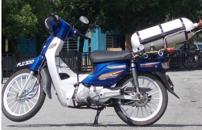
Figure 15: This motorcycle has been converted to operate on CNG and can travel 200km for RM4 (about 1 USD) of fuel (Source: Author, 2016).
