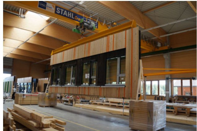
A high degree of prefabrication of components ensures planning reliability and profitability (prefabricated timber frame wall)
