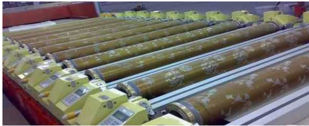
Image no. 6: Rotary Screen Printing [Source: Retrieved from http://textilelearner.blogspot.in/2012/01/rotary-screen-printing-machine-working.html ]
