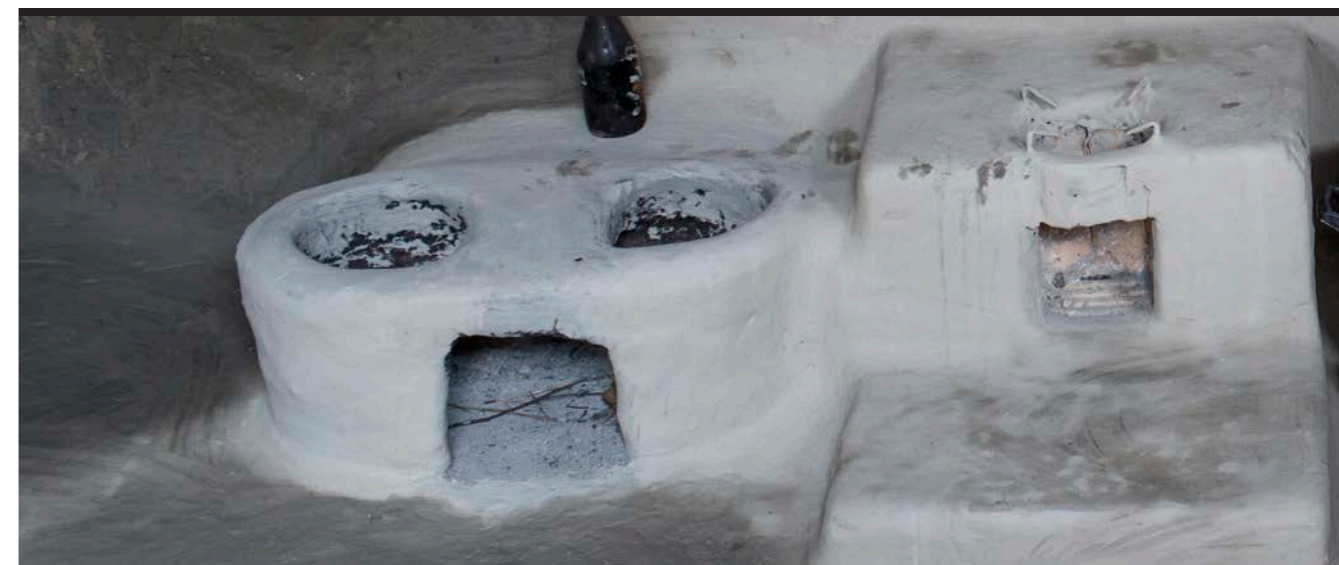
Picture 1: Traditional Indian Two-burner Cookstove (left) and Fixed Improved Single-burner Cookstove (right)
